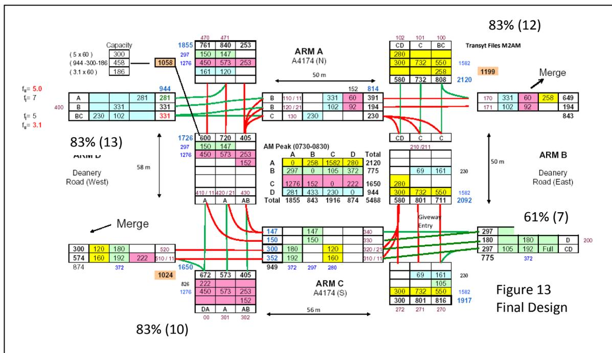
The above final design and optimum operational timings were produced using the JCT LinSig software. The Lane/Flow Diagrams illustrated above use the Microsoft Excel program. This is purely for teaching purposes. Lane/Flow diagrams are created automatically by the JCT LinSig software as you model build and explore various design options.
